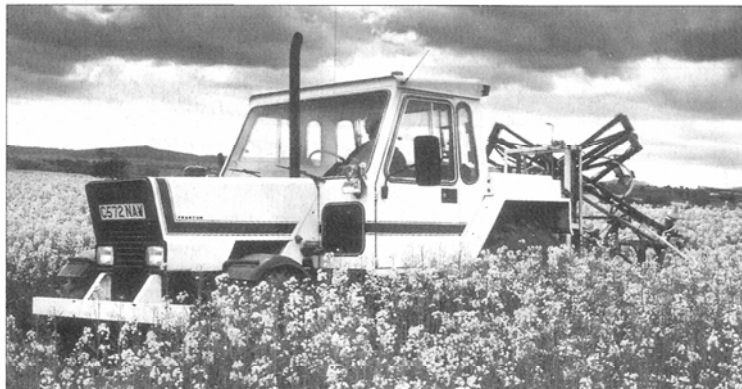
The lighter weight 4WD Trantor 'transport-first' tractor just completing work in the field and returning to the water source at speeds far in excess of that possible with 'ploughing-first' tractors.
