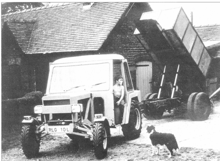
The prototype 41 kW Trantor at harvest time in 1973; designed to pull a bigger trailer than a Land Rover but travel at Land Rover road speeds
